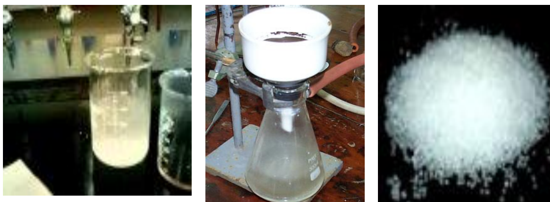
Figure 4.5. Preparation of adipic acid in a school's chemical laboratory. The white (milky) solid crystals can be easily separated and dried.
