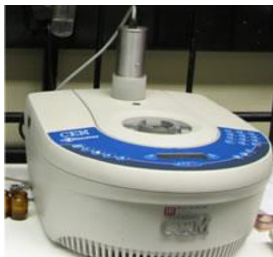
Figure 4.8. New equipment appeared in the market for microwave irradiation reactions with special reflux condensers and digital indicators.
